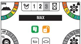
Figure 3. shows Zone 3 "Heavy Duty" Factory Configuration.
